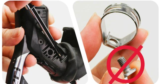
4. Install the replacement Clamp Bolt into the Handlebar Clamp and engage the Clamp with the Lever Body, aligning the Clamp Bolt with the Clamp Nut
