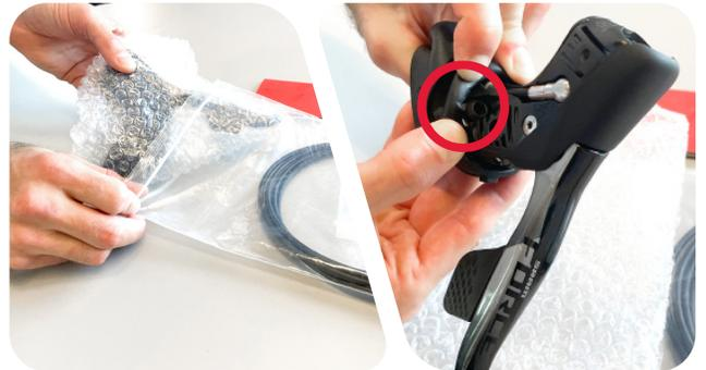
3. Loosen the Lever Clamp Nut with a 5 mm hex wrench until the Handlebar Clamp and Clamp Bolt are released from the back of the Lever Body.
